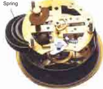
Spring Flat spiral spring of a mechanical clock.
